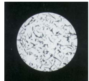
Cast (Gray) Iron Pipe
