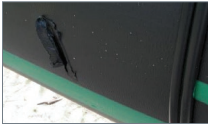
A scratch or ding (shown here) would disqualify this HDPE from installation.
